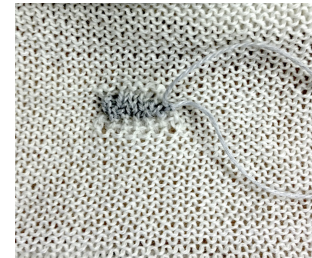
Figure 3: conductive yarn knitted on a second needle bed and linked with non conductive yarn
