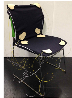
Figure 1: Backside of the chair cover, all sensors attached, before connecting them to other hardware.
